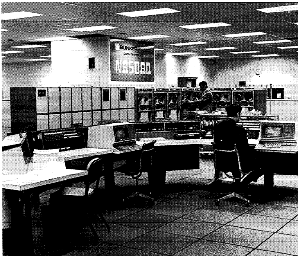
NASDAQ COMPUTER CENTER: In this area, two Univac 1108 computers receive and process information from NASDAQ market makers.
